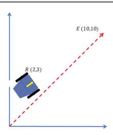
The distance of the robot to the trajectory is computed using the dot product:
